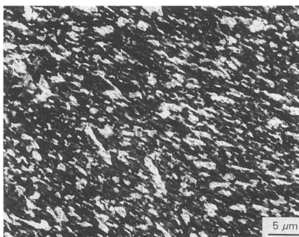
Figure 5 Transmission electron micrograph of 40/60 ASA/PBT blend showing the dispersed ASA phase. The continuous dark phase is PBT.
